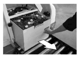
13.Lower the cart's battery stop bar by pulling up on the handle. This will keep the batteries from rolling off the cart when moving.
