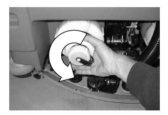
10.ES™ mode (option): Remove the solution tank drain hose cap while holding the hose up, then slowly lower the drain hose to the floor drain.
