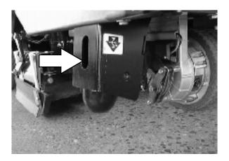
The rear tie-down locations are on the rear corners of the machine.
