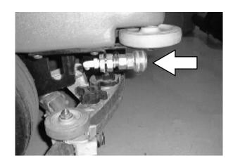
7. Assemble the *power wand*, and attach the other ends of the solution and vacuum hoses to the *power wand*.
