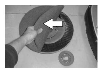
10. Replace the center disk to secure the pad in place on the driver.
