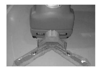
7. Remove and refasten the *QuickMop* <sup>™</sup> head covers with the easy to remove snaps. Remove the head covers to rotate, shake and clean at regular intervals.
