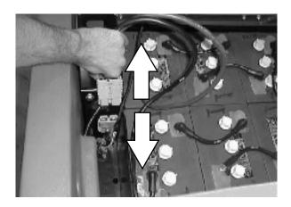
Push the battery cart to the right hand side of the machine. Line up the battery cart locks and the tabs on the machine. Push the battery cart forward.
