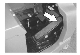
3. Press the *scrub switch* to start the scrubbing operations. See the SCRUB SWITCH section of the manual.
