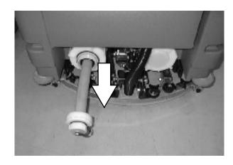
11. ES™ mode (option): Lift the tank cover and flush out the solution tank with clean water. Rinse the filter at the bottom of the solution tank and the pressure switch near the top of the tank.
