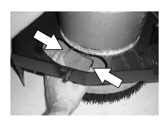
15. Close the side squeegee, and secure in place with the washer and cotter key.
