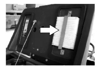
Check the vacuum fan inlet filter daily. Remove the filter bracket to remove and clean the inlet filter. Clean inlet filter with a damp cloth or hose when dirty. Allow filter to dry completely before replacing it into machine.
