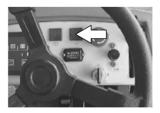
14. Press the *squeegee switch* to stop the vacuum system and raise the rear squeegee.
