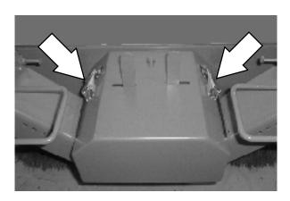
5. Pull the release lever to raise or lower each side of the  $QuickMop^{\mathsf{TM}}$ .
