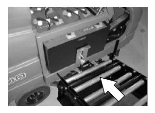
6. Lock the battery cart to the machine by closing the battery cart locks around the machine tabs.
