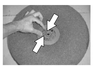
9. Flip or replace the scrub pad, center the scrub pad on the pad driver.
