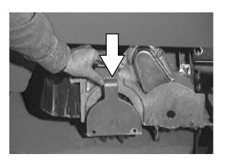
B. While holding the flat end of the idler shaft with a wrench, loosen the mounting screw on the outside of the idler door.
