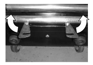
15. Release the battery cart floor lock. To release floor lock, step down on the right side of floor lock.
