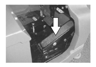
Forward: Press the top of the *directional pedal* with the upper part of your foot.
