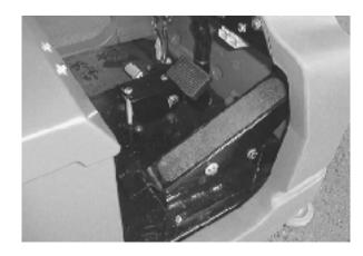
3. Press the brake pedal to stop the machine.
