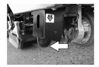
Jack up the rear of the machine from underneath the rear corners. Use a piece of wood between the jack and the frame to distribute the machine weight load.
