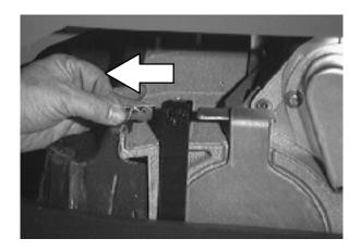
4. Push downward on the mounting spring and idler door until the top of the door releases from the scrub head. Pull the bottom of the door outward, then pull the idler door and idler plug off the brush.
