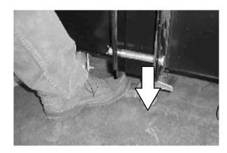
8. Adjust the battery cart rollers before rolling out the batteries. The battery cart rollers must be the same height as the machine battery rollers.
