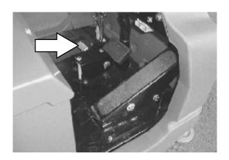
5. Access the recovery tank drain hose by loosening the retaining ring and then pulling the hose out.
