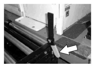
12. Grab the battery case slot and pull the battery case onto the battery cart.
