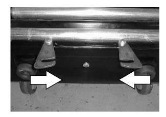
7. Set the battery cart floor lock by stepping down on the left side of floor lock.
