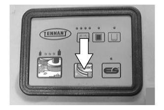
10. Press the top of the *power wand switch* to turn the power wand on.
