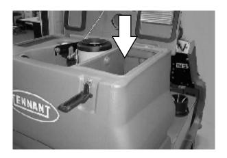
9. ES<sup>™</sup> mode (option): Access the solution tank drain hose by loosening the retaining ring and then pulling the hose out.
