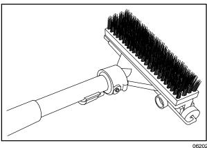
If the *power wand* is hard to push or is not picking up the solution very well, adjust the roller wheels on the tool by turning the black adjustment knob.
